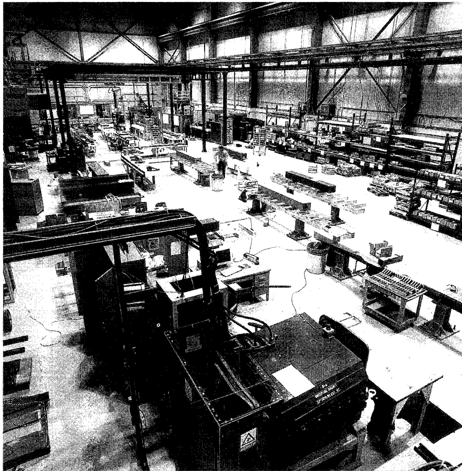
A view of Fermilab's permanent magnet factory, with the ferrite brick magnetizing station in the foreground and several magnets under assembly on the central floor.
